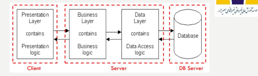
$\,\circ\,$  Each layer can potentially run on a different machine
